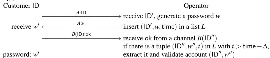
In this protocol, time denotes the clock value and  $\Delta$  denotes a maximum time delay after which a password request session expires on the server side if not completed. After the protocol completes, the customer can authenticate through the  $A$  link by using a password.
